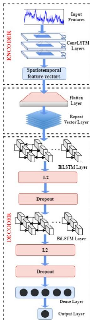
**Figure 4. Proposed ConvLSTM-BiLSTM based Encoder-Decoder Architecture**
